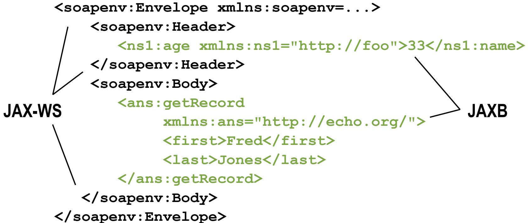
The diagram illustrates the division of work between JAX-WS and JAXB. On the left, the text "JAX-WS" is associated with the entire XML envelope, header, and body. On the right, the text "JAXB" is associated with the namespace declarations (`xmlns:ns1="http://foo"` and `xmlns:ans="http://echo.org/"`) and the `getRecord` message. Arrows point from the labels to their respective parts of the XML code.
